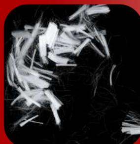
ConFib Microfibers & Macrofibers are engineered from 100% virgin polypropylene, precisely designed in a micro-fibrillated form to enhance concrete performance. Through this, effectively minimize the risk of cracking due to plastic shrinkage and settlement by creating a network system in concrete. These fibers go a step further, enhancing the overall durability and toughness of the concrete, making it a more valid construction material.
